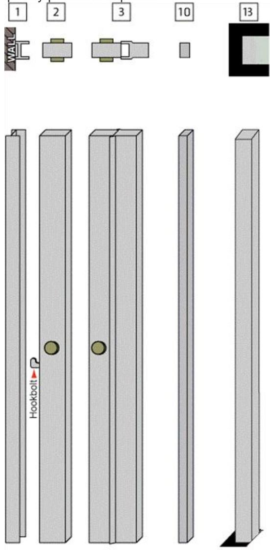
**1** Wall Channel - A full height extruded piece of aluminum that the Lead Post fits and locks into. This Channel is secured permanently to the wall.
