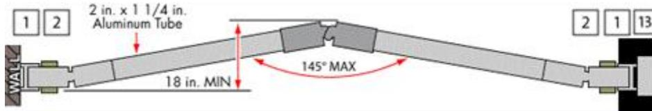
Typical layout connects to wall at one end and mounting tube at other end. Layout can have multiple sections.
